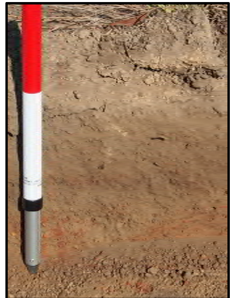
Figure 28: Profile of Trench 11 showing hard lateritic soils close to the surface
