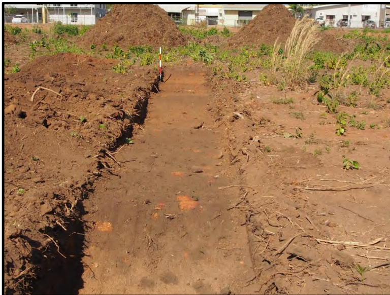
Figure 27: Trench 11 illustrating the shallow soil above the uneven laterite bedrock
